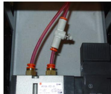
With the valve and cylinder connected, the last step in the pneumatic plumbing is to run the supply line (P Port). To do so, simply take the remaining 1/4" airline fitting (1/4" NPT threads) and connect it to your air compressors 1/4" NPT female threaded fitting (not supplied). Next take
