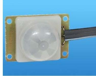
Note: A PIR (Passive Infrared) sensor is **NOT** a prop controller. A PIR is a signal generator that creates pulse signals (rapid on and off, approx .5 sec) that are sent to a receiving automation controller such as an SD Keybanger, Efx-Tek Prop 1 Microcontroller, HE Animation Maestro, or Terror by Design UDT2 or Puppetmaster.
