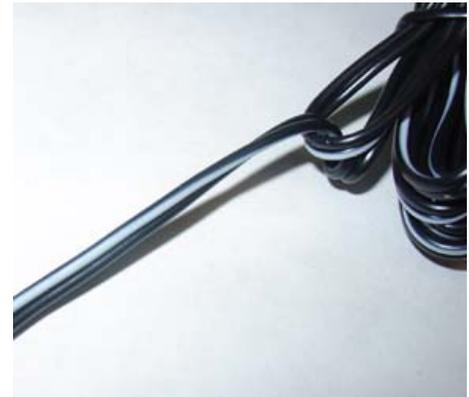
With the power supply un-energized, take the power cord (running from the power supply to the valve) and separate (spilt apart) the two wires about a foot from the power supply. As a precaution, all wiring should be kept as far from the valve and water as possible. Once split you should be left with a solid black wire and a black wire with a white stripe.
