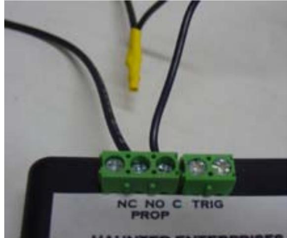
This will complete the circuit, and the controller will “close” the circuitry loop, per your program using a PIR (passive infrared) sensor, push button trigger, or switch mat (only connect ONE trigger at a time!).
