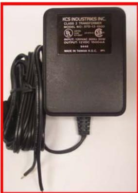
The 1500 mA power pack is sufficient to drive the Rev 2 IOGeek and up to 1000 mA of external 12 VDC hardware.
