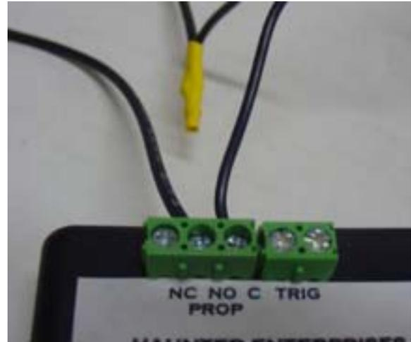
can connect the first (common) wire coming from the power supply into the “C” (constant) terminal. Next connect the wire running to the valve on the lifter into the “N/O” (normally open) terminal.
