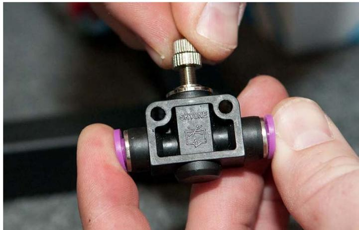
In regards to displaying your prop, never use this mechanism at more than 120PSI. We recommend 80PSI which will prolong the lifter and prop life and avoid possibly hurting an innocent viewer. Also never use this mechanism in close vicinity (arms reach) of viewers. All of our pneumatic parts are rated to 120PSI, adding more will cause them to fail and begin leaking air or possibly a release of the tubing (never try and “catch” a loose/whipping pressurized airline).
