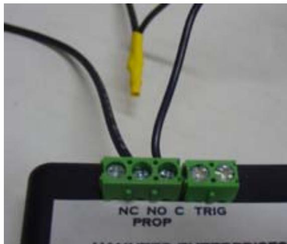
This will complete the circuit, and the controller will “close” the circuitry loop, per your program using a PIR (passive infrared) sensor, push button trigger, or switch mat (only connect ONE trigger at a time!).
