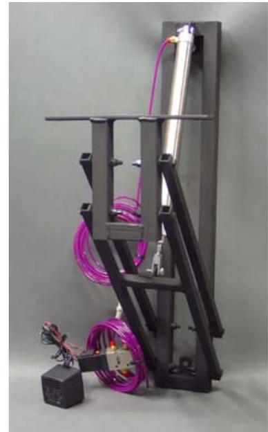
The barrel lifter was designed to be used in conjunction with a standard steel 55 gallon barrel and can be used completely submerged in water. Please note, if using the barrel lifter in a submerged state, please keep all electronics as far away as possible. It is also recommended to oil the cylinder rod periodically with pneumatic tool oil, and store the barrel and lifter completely drained and dry.
