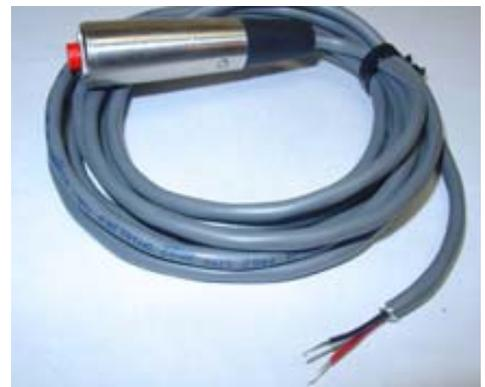
the wire coming from the power supply to the red wire, and the other cut side (the wire that's running to the valve) to the black wire. We strongly recommend soldering these connections, then covering all of the bare wire with heat shrink tubing and or wrapping with electrical tape.
