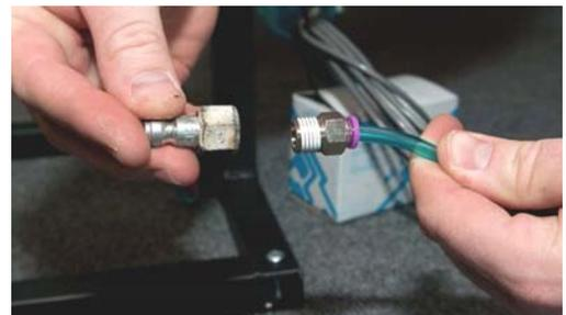
air supply (the cannon will fire at this point automatically) and allow the cannon to drain. If the leak is heard at the tubing, push the tubing further into the fittings and or tighten the fitting a 1/2 turn (or possibly more – but DO NOT OVERTIGHTEN). Re-connect your air source and re-test.
